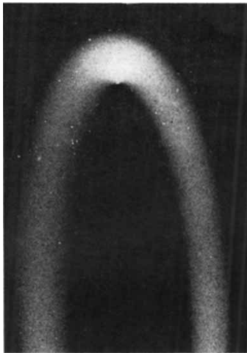
Fig. 3. Microradiograph of a bent nylon monofilament (0.38 mm.). Aluminum target, 15 kv. The long axis of the filament in Fig. 2 has been rotated slightly so that the arm which appears larger in diameter is closer to the target than the other.
